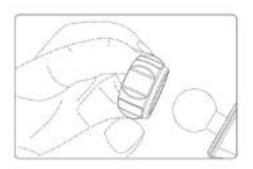
Unscrew the fixed nut and choose the air vent clip, then set the ball in the fixed nut. Fasten the nut into the spherical top and push the nut forcibly into the round hole at the back of the car phone mount.
