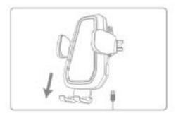
4. Plug the Micro-USB charging cable into the power interface. Pull down the LED bracket and the height adjustment area appears. Customers can adjust the LED bracket's height according to their cell phones' size.
