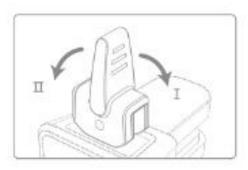
3. Fix the automatic wireless car charger on the suitable place of air vent. There are two gears in the clip, and left or right can be selected. It is recommended that the thick wind leaf choose one " I " and thin choose two " II ".
