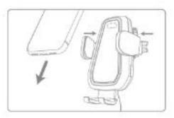
5. Put the mobile phone in the car phone mount to trigger switch. The arm lock automatically clamps the mobile phone and starts the wireless charging. At the same time, the LED bracket lights up. If there is no respond with the arm lock, tap the upper part of the phone screen.
