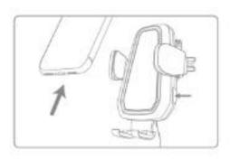
Pressing any button on the edge shortly, the arm lock stretches automatically after using. You can take out your phone from the mount easily as shown in the picture.
